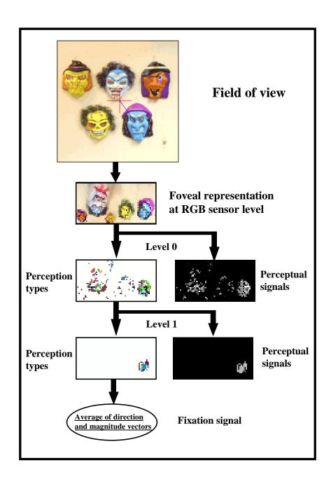
Figure 5: The two level colour processing control system used in our experiments. The outputs from these levels, of the magnitude and direction to the target, define the input to the highest level (fixation) control system.
